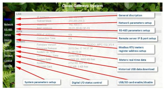
Note: After each setup, please do not forget to "save" the setting. The setting will be effective after WPC-132 "reboot" successfully.
